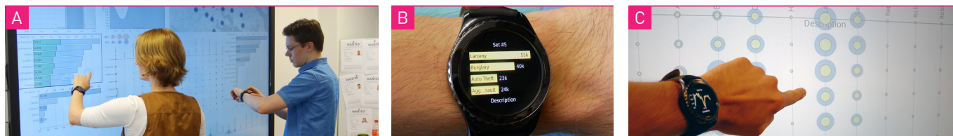
Figure 1. Visual data analysis using large displays and smartwatches together. Cross-device interaction workflows discussed in our conceptual framework allow for an interplay between these two types of devices. For instance, multiple analysts can extract data from views on a large display (left) to their smartwatches (middle) and compare the data on other visualizations distributed over the large display by physical movements followed by direct touch (right) or remote interaction. This pull/preview/push interaction metaphor can be extended to many visualization tasks. The watch enhances the large display by acting as a user-specific storage, a mediator, and a remote control, and further aids multiple users working in concert or by themselves.
