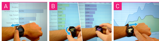
Figure 9. (a) Pulling, (b) previewing, and (c) pushing of sets.
